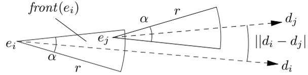
**Fig. 2.** The front regions of  $e_i$  and  $e_j$  as wedges of edge length  $r$  and apex angle  $\alpha$ . Entity  $e_j$  is in front of  $e_i$ . The entities are heading into directions  $d_i$  and  $d_j$ , respectively. If  $\|d_i - d_j\| \leq \beta$  then  $e_i$  follows  $e_j$ .
