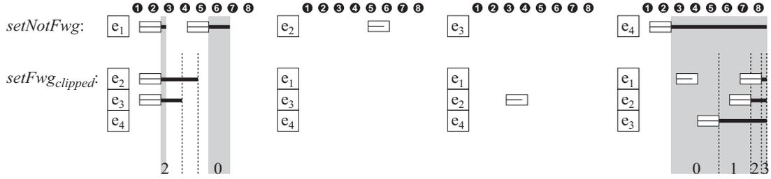
**Fig. 8.** Illustrating the parallel scan approach. The shaded region indicates how the  $SetNotFwg$  intervals are used as a mask. The numbers indicate the number of active  $SetFwd$  intervals.
