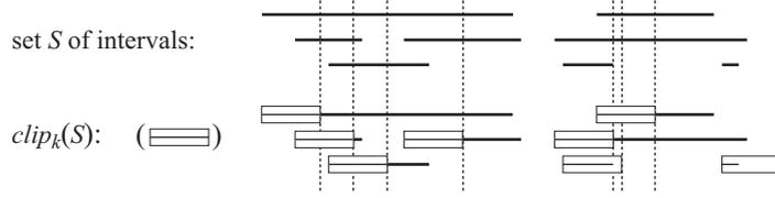
**Fig. 6.** The set  $S$  of intervals on the real line and the results after applying the  $clip_k$  operation. For the  $clip_k$  operation, the length of the interval in parentheses determines  $k$ .
