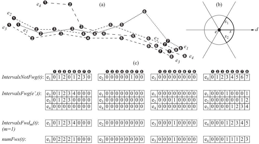
**Fig. 1.** (a) A set of 4 entities moving from left to right over 7 unit-time-intervals, i.e. over 8 time-steps. (b) Illustrating the definition of the front-region as the disc-segment within bold lines. (c) The follow-arrays of the four entities, where we use the front-region as depicted in (b) and  $\alpha = \beta$ .
